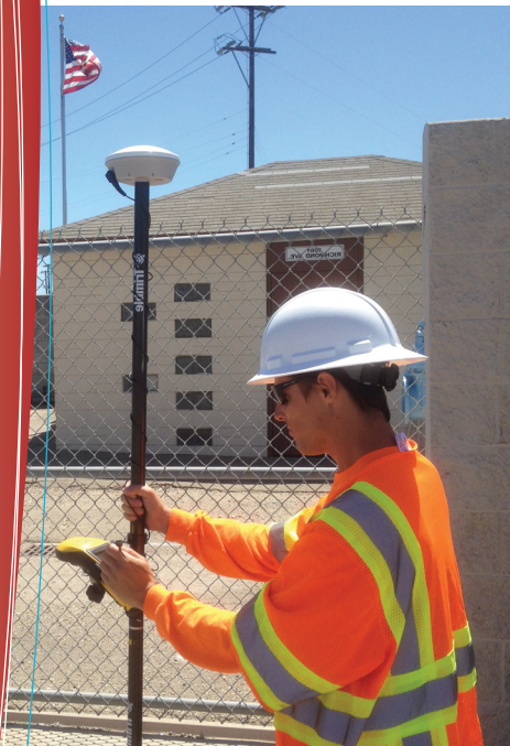
Data collection using Trimble GeoExplorer 6000 GPS unit with attached Tornado antenna
